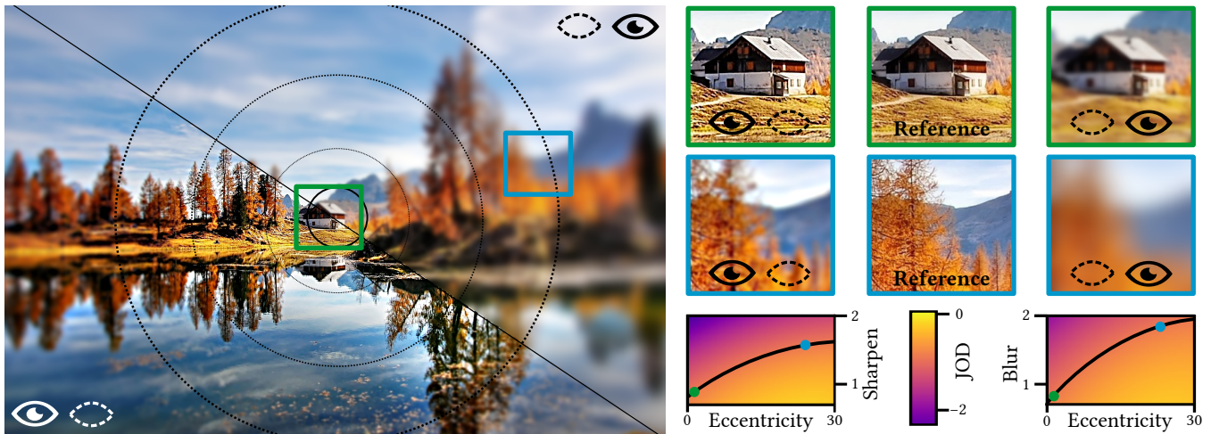
Fig. 1. We present dichoptic foveation, a new paradigm to parameterize quality degradation of dichoptically-rendered stimuli in stereoscopic displays like virtual reality. Particularly, we apply Gaussian blur on the stimulus of one eye (right inset images here), while the other eye’s stimulus is processed by a simultaneous sharpening routine (left insets). This is guided by our computational model (see heatmaps), which is built on psychophysical data. Dichoptic foveation has direct implications for better quality-to-compute ratios in foveated rendering. Image by kordi_vahle from Pixabay.
